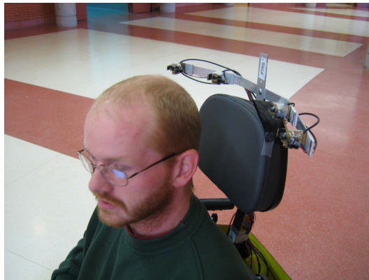
Figure 8.3: Photo of possible attachment of the disclosed HMI on a wheelchair.
