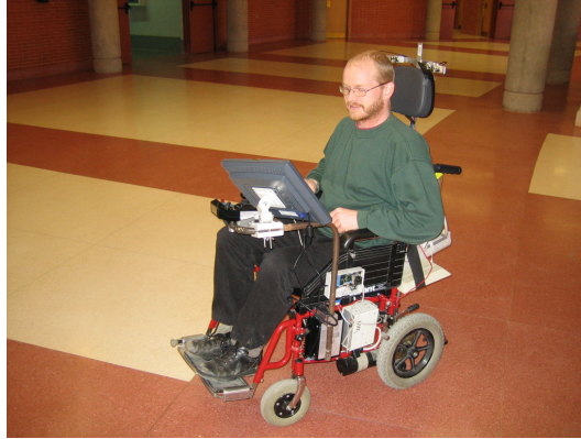
Figure 8.2: The sensors attached to the head rest piece of the SIAMO wheelchair.
