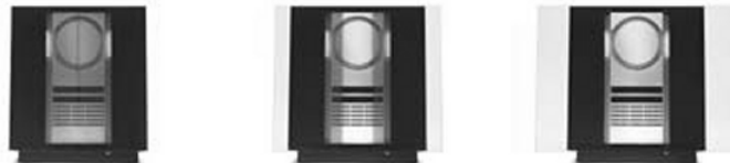
Figure 3.3: The sliding doors in the BeoSound Overture is activated by the presence of a hand. The hand is detected by infrared sensors behind the black panels in each side of the CD player. Source: B&O web site.
