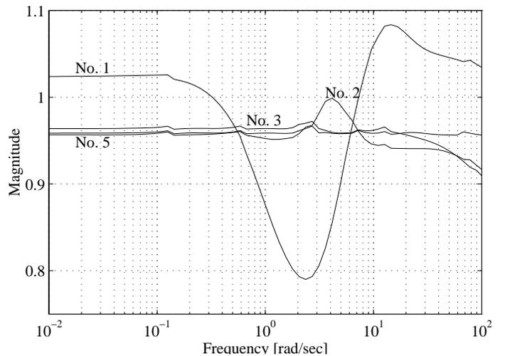
Figure 3: Upper  $\mu$  bound for step 1 (the optimal  $\mathcal{H}_\infty$  controller), 2, 3 and 5 in the  $\mu$ -K iteration for the pump system example.
