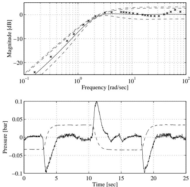
Figure 4: Results from applying  $\mu$ - $K$  iteration on the water supply system.
