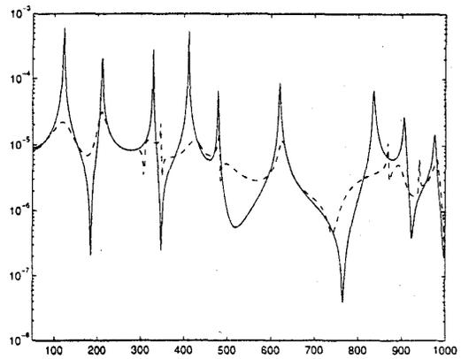
Fig. 5. Frequency response to point force
