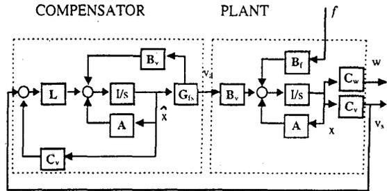
Fig. 4. Block diagram of the actively controlled system.
