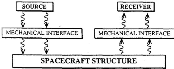
Fig. 1. Microvibration propagation path.
