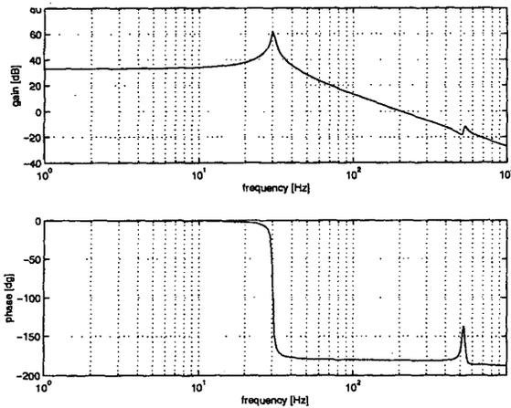
**Figure 6:** Focus actuator model (without anti aliasing filter).
