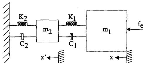
Figure 1: Translational diagram of the optical pick-up.
