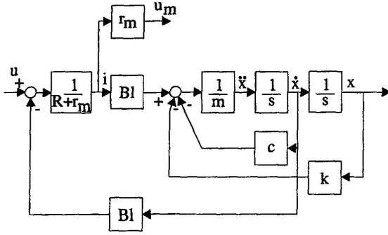
Figure 3: State space diagram of  $F(s)$  (reduced order).
