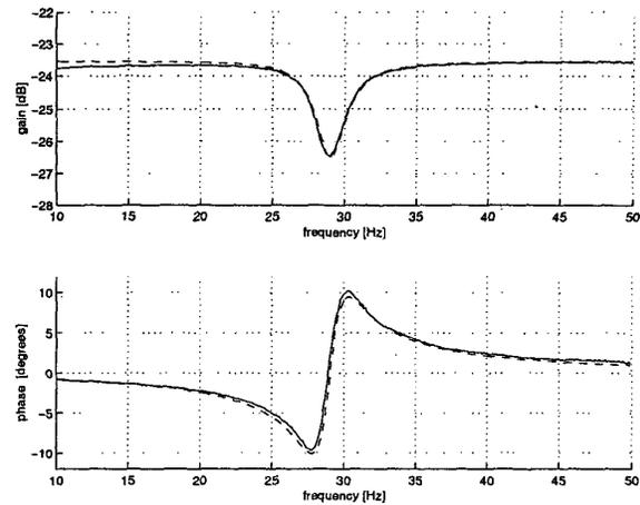
**Figure 5:** Measured (solid) and fitted (dashed)  $F_{12}(s)$  transfer function.
