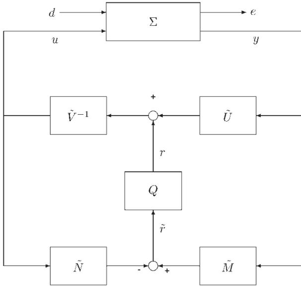
Figure 2. Controller structure with parameterization.
