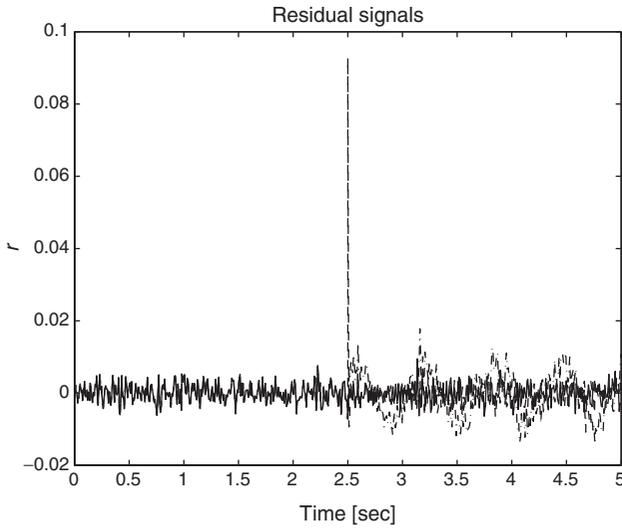
Figure 8. The residual signal  $r$  of the servo system. The solid line is the output for the nominal system, the dashed line is for the system with an additive fault and the dashdot line is for the system with a parametric fault.
