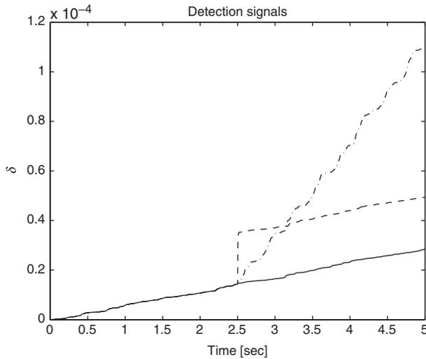
Figure 9. The detection signal  $\delta$  for the servo system. The solid line is the output for the nominal system, the dashed line is for the system with an additive fault and the dashdot line is for the system with a parametric fault.
