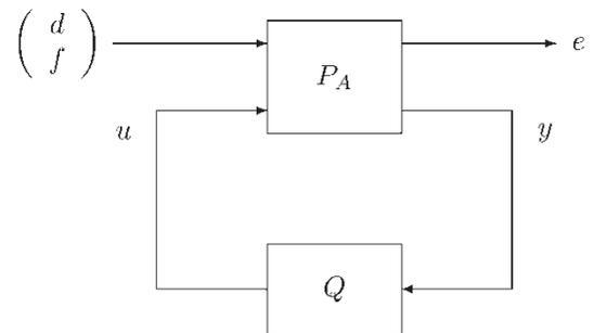
Figure 5. The standard setup for design of  $Q$  for systems with additive faults.
