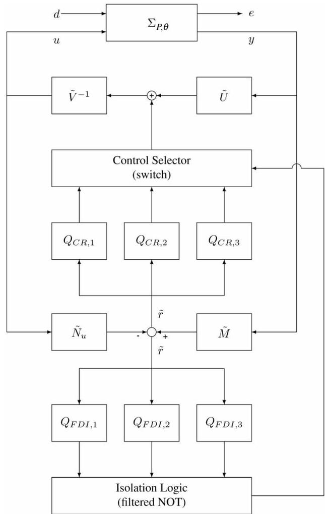
Figure 3. Fault tolerant scheme with three potential parametric faults. The residual signal is used both for isolation and for feedforward in the fault handling.
