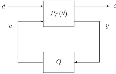
Figure 6. The standard setup for design of  $Q$  for systems with parametric faults.
