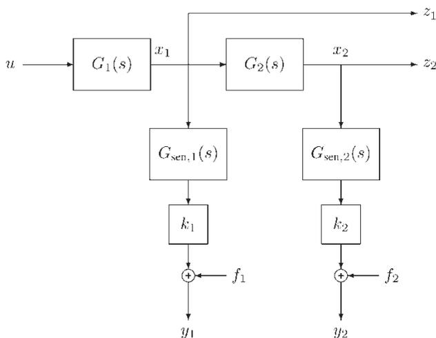
Figure 1. Block diagram of a dynamic system including two sub-systems and two sensors.
