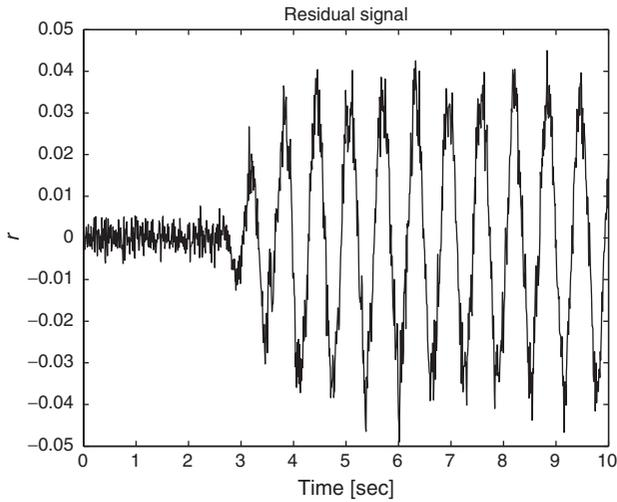
Figure 11. The residual signal  $r$  of the servo system.
