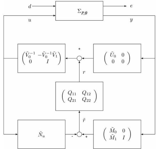
Figure 4. Block diagram for controller with a  $Q$  parameterization. Note that the nominal controller does not use the measurements employed after reconfiguration.
