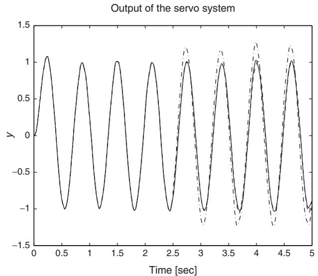
Figure 7. The time response of the output  $y$  of the servo system. The solid line is the output for the nominal system, the dashed line is for the system with an additive fault and the dashdot line is for the system with a parametric fault.
