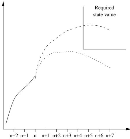
Fig. 3. Illustration of situation where a specific output value is required to be reached with a given time. This figure shows two possible future behaviors of the system, where one reaches the required value in time and the other do not.
