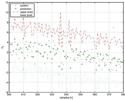
Fig. 6. Plot of the predicted and “real” output  $T_s$ , without linear interpolation.
