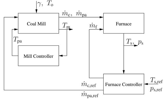
Fig. 4. Illustration of model structure
