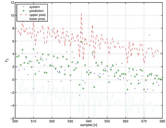
Fig. 9. Plot of the predicted and “real” output  $T_s$ .
