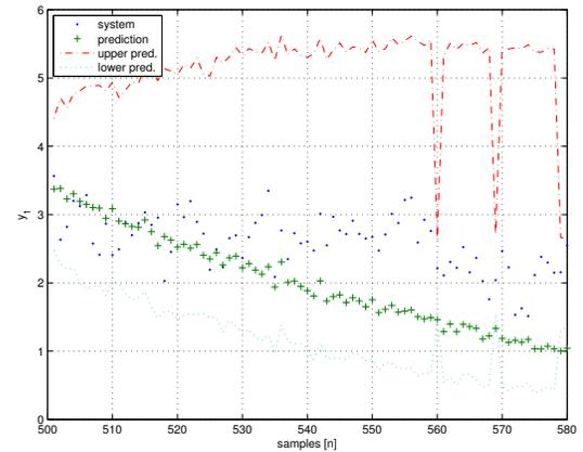
Fig. 5. Plot of the predicted and “real” output  $T_g$ , without linear interpolation. The three spikes at the bounds at time 560, 570, 580 is due to change operating points.
