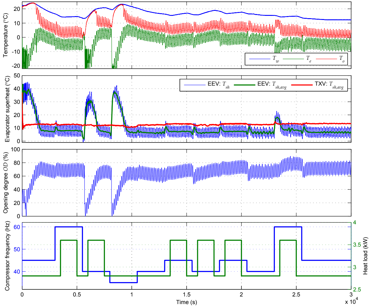
Fig. 10. Test of the harmonic controller on the refrigeration system. The load in the bottom plot is approximately the heat applied to the water tank. The same time scale is used for all four plots. The average superheat achieved with a TXV in a similar test without harmonic control is shown for comparison.
