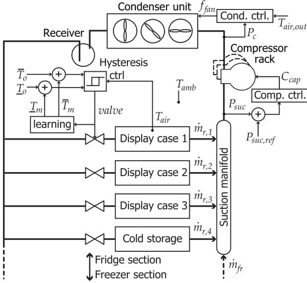
Fig. 4. Overview of supermarket refrigeration system model with multiple display cases and a cold storage room. The freezer section is simulated by an additional mass flow  $\dot{m}_{fr}$  and controllers are used to regulate pressures and temperatures as indicated. Only one of the valve hysteresis controllers are shown in the figure.
