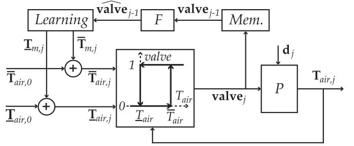
Fig. 7. Relay feedback controlled system  $P$  with adaption of the thresholds using a learning-based approach. The trial domain is denoted  $j$ .
