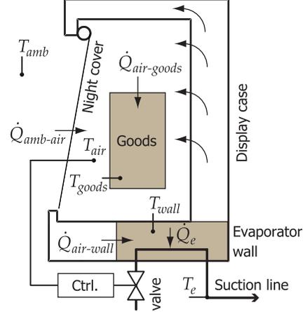
Fig. 5. Open shelf-type display case model with night cover.
