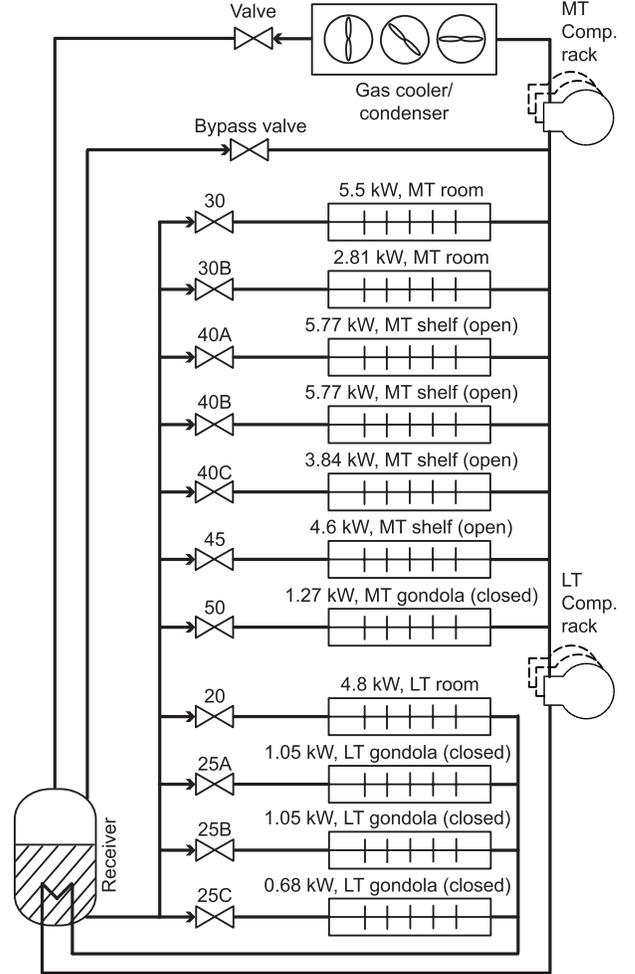
Fig. 1. Simplified schematic of the medium size supermarket refrigeration system. The numbers on the valves are used as reference.
