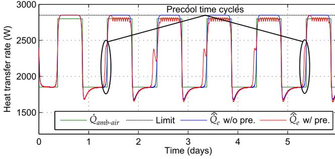
Fig. 10. Simulation results with and without precool using the simple example model with a max load of 2.8 kW and an upper limit on  $\hat{Q}_e$  of 2.85 kW.
